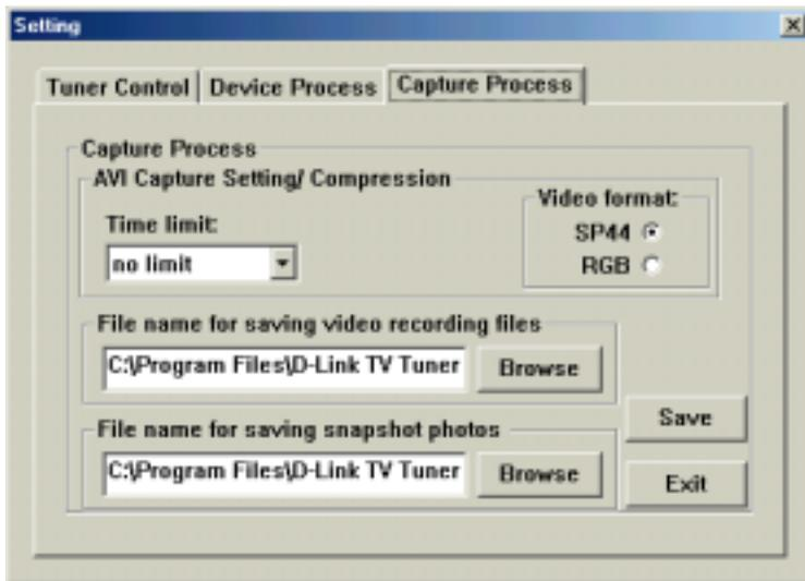
The “**Time limit**” drop down box allows you to select the recording time limit from 30 seconds up to 120 minutes or no limit. All files are saved in AVI format. You can also change the **Video Format** to SP44 or RGB.
