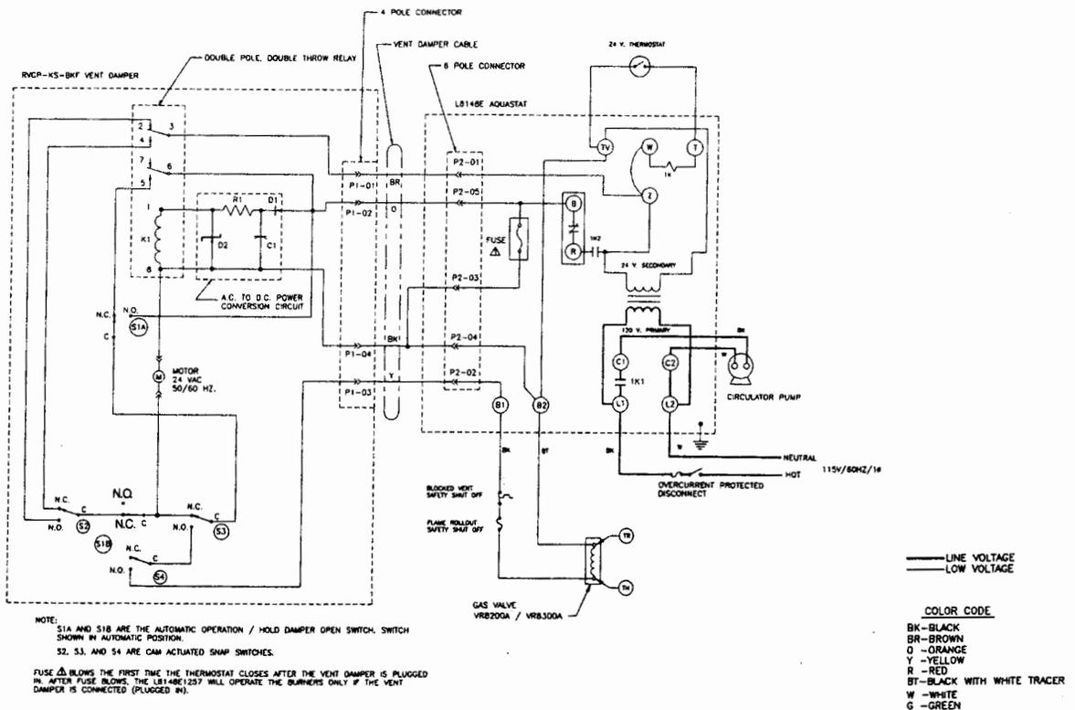
**IF ANY OF THE ORIGINAL WIRE AS SUPPLIED WITH THIS APPLIANCE MUST BE REPLACED, IT MUST BE REPLACED WITH TYPE 105° C THERMOPLASTIC WIRE OR ITS EQUIVALENT.**
