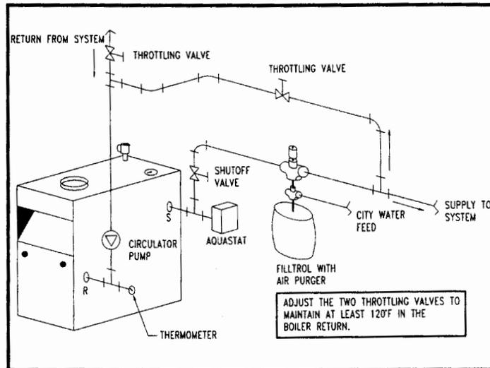
**BYPASS PIPING REQUIRED FOR HIGH MASS (LARGE WATER CONTENT) SYSTEMS**
