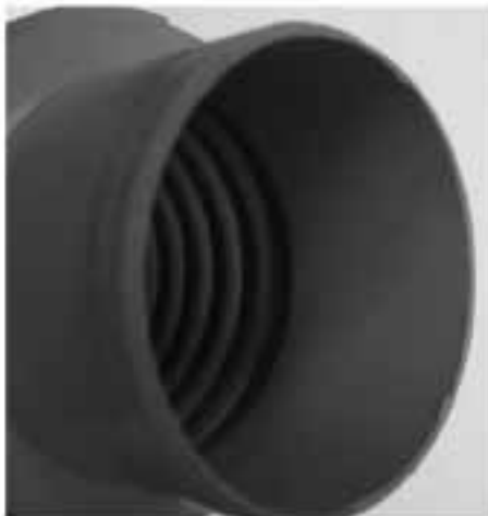
C: Liner Bottomed Out in Adaptor
