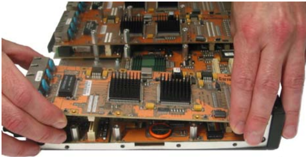
Figure 3.5.3b: Removing a 6KPM Card
