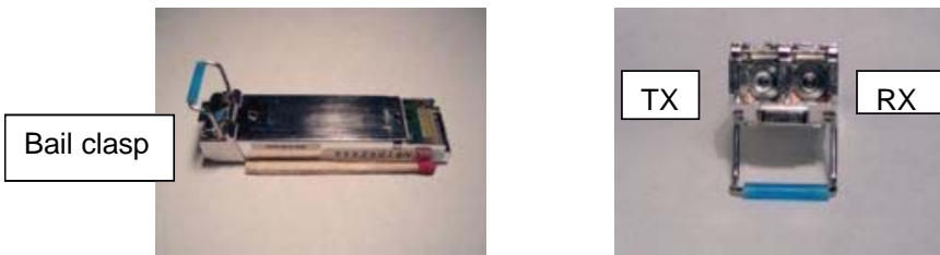
Side View ---Duplex LC connector -- Front view
