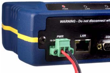
Figure 2. Power Connector (Polarity: Left +, Right –)
