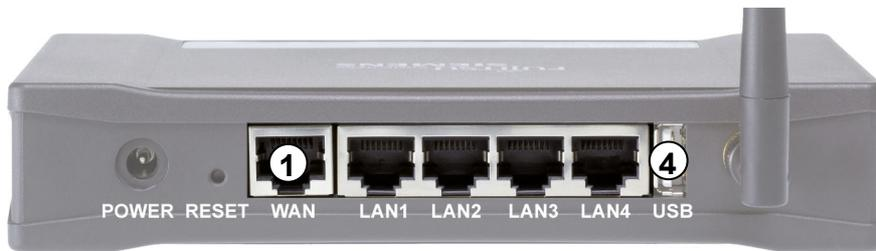
Connect the CABLE Modem to the WAN port. Additional networking devices like network printers, servers or scanners can be plugged into one of the free LAN ports and will be integrated in the IP segment of 192.168.1.X.
