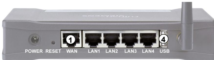
Connect the ADSL Modem to the WAN port, otherwise the PPPoE session cannot be established and therefore the Internet service cannot be opened. Additional networking devices like network printers, servers or scanners can be plugged into one of the free LAN ports and will be integrated in the IP segment of 192.168.1.X.
