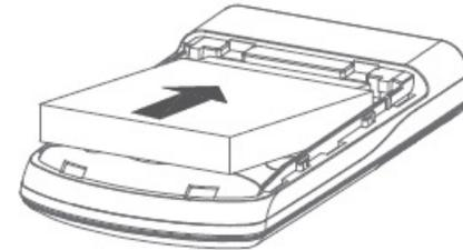
3. Replace the battery cover and gently press down while sliding the cover until it locks into place.
