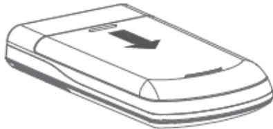
2. Insert the battery by lining up the gold contact points on the battery with the gold contact points in the device's battery compartment. Then press down gently until the battery is seated.
