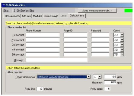
Figure 2-7 Setting dialout phone numbers and alarm conditions
