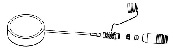
Figure 3-3 Protective connector shell pieces for the in-street antenna
