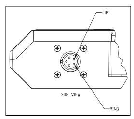
Figure 1-4 2103 Modem Cable Connector
