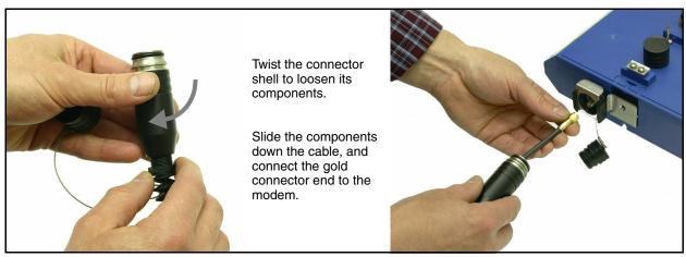
Figure 4-6 Connecting an antenna to the 2103G
