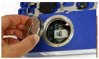
Figure 4-1 Accessing the SIM card on the bottom of the module
