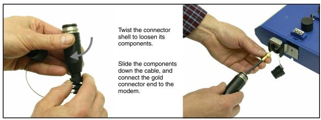
Figure 3-4 Connecting an antenna to the 2103C
