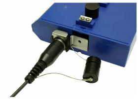
Figure 3-5 Antenna connected to the 2103C modem.
