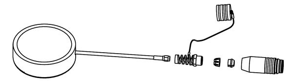
Figure 4-5 Protective connector shell pieces for the in-street antenna
