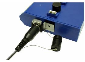
Figure 4-7 Antenna connected to the 2103G modem.
