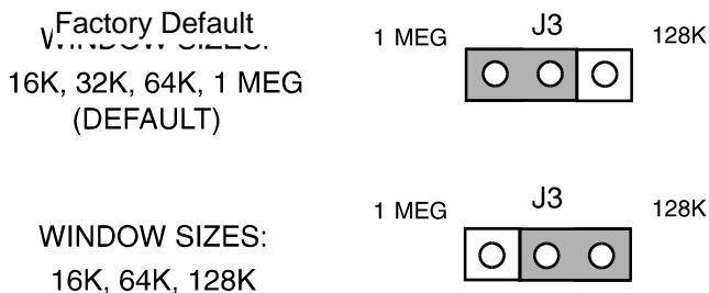
Figure 2-13 Window Group Select Jumper Plug Settings
