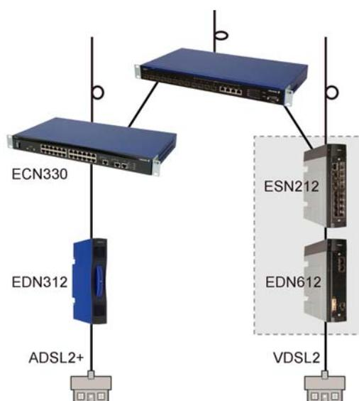
In essence, VDSL2 can be added to an existing ECN330-based site. This is done by connecting an ESN410/ESN212 to an uplink port of the ECN330 and optionally adding additional fiber uplinks to the new switch for traffic aggregation. The IP DSLAMs below the ESN410/ESN212 will be handled by the EMP in the ECN330 and hence “piggy-bag” on the existing installation.
