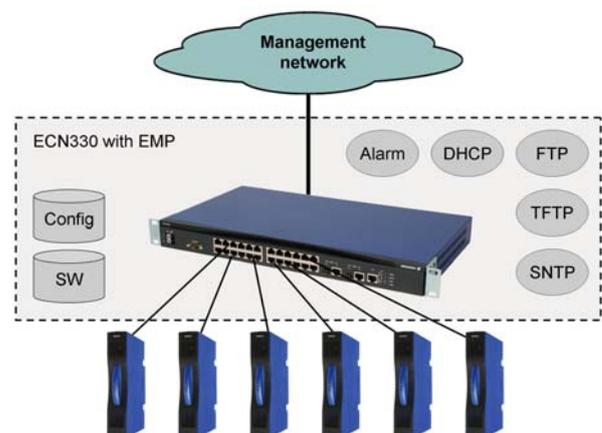
In this way, there is only one management interface and one static IP address. For provisioning, the EMP is managed via standard MIBs, and for system maintenance via EDA SNMP MIBs. All SW images and configurations are stored in local non-volatile memory to secure full operation, even if access to the management system is unavailable.
