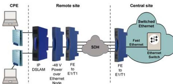
EXN104 supports up to four 120 Ω E1/T1 ports each with a speed of 2 Mbps. EXN104 conforms to ITU-T G.703 on the LSA® interface and is fully manageable via SNMP from PEM.
