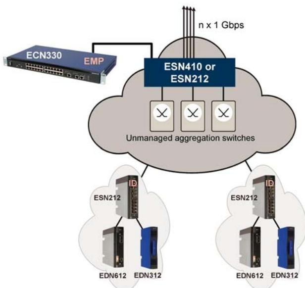
The flexible topology support is particularly powerful for VDSL2 deployment in scenarios where telecom operators already have access aggregation switches in place, with non-Ericsson equipment.
