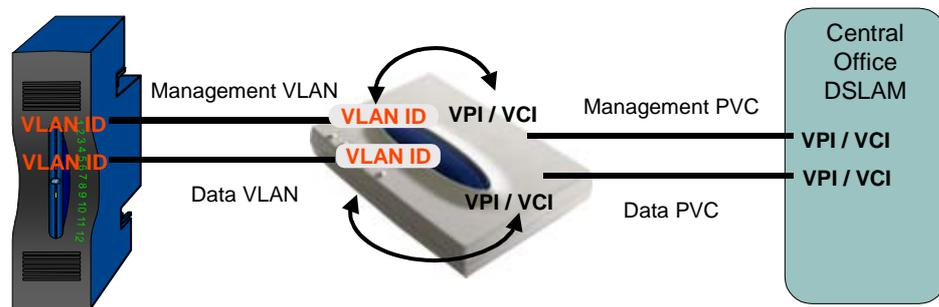
Figure 4 Configuration of the CPE Modem
