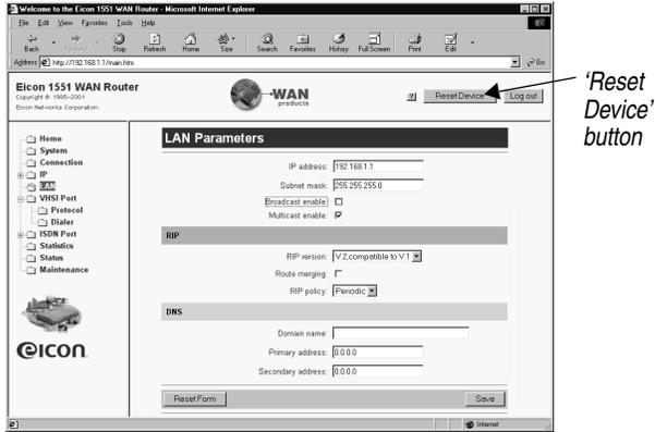
Once you have reset the device, test that you have access to the remote device using your WAN application. You can also ping the remote device to which you are attempting to connect.
