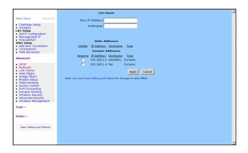
New IP Address: Enter the IP Address.
