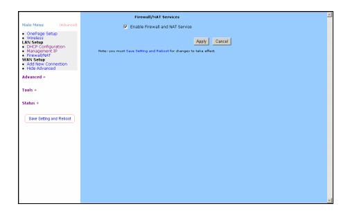
*Firewall/NAT Services:* Select Enable to turn on the Firewall/NAT Service. *Apply:* Click Apply to save the changes.
