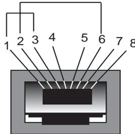
To connect the hub to another hub, switch, bridge or router, use a swap cable swapping pins 1 to 3, 2 to 6, 6 to 2, and 3 to 1.
