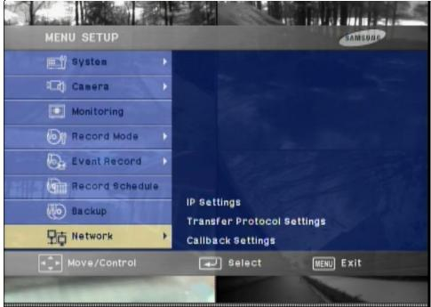
4) You should use the cursor buttons to scroll over to IP SETTINGS and then press the ENTER button
