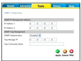
Use SNMP to configure system features for proper operation, performance monitoring, and detection of potential problems in the Router or network.
