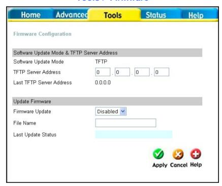
You can update both the software and firmware of the Router. Please check the D-Link Support site for firmware updates at <a href="http://support.dlink.com">http://support.dlink.com</a>. You can download firmware upgrades to your hard drive from the D-Link support site.
