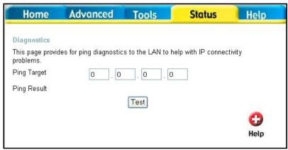
The Diagnostics window allows users to test the functionality of the router by executing a ping test. Enter the IP address of the Ping Target and then click **Test**.
