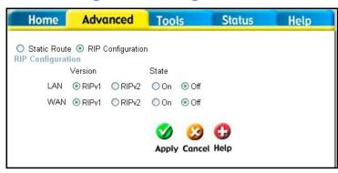
LAN RIPv1 Select RIPv1 or RIPv2 for use by the router on your LAN.
