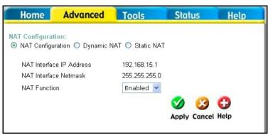
NAT Interface IP Address This field displays the current IP address of the LAN side of the router. All IP address that are translated by the router will be in the same range as this IP address.
