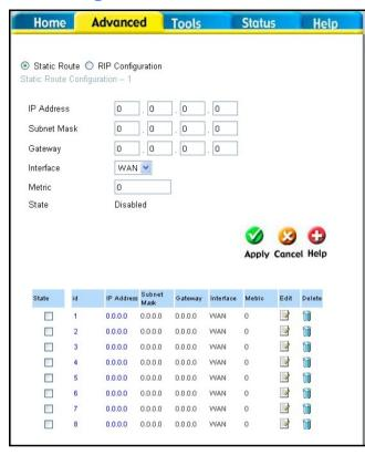
Enter the IP Address of the subnet or device where packets are to be routed Subnet Mask Enter the subnet mask corresponding to the IP address entered above. Gateway Enter the IP address of the gateway used for packets that are to be routed to the IP address entered above. Interface Select the WAN (Internet) or LAN interface. Enter the number of hops (the number of routers) that packets Metric
