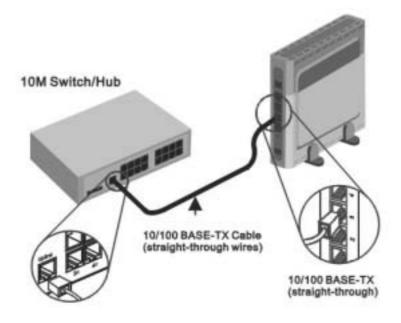
If you wish to reserve the uplink port on the switch or hub for another device, connect to any on the other MDI-X ports (1x, 2x, etc.) with a crossed cable.
