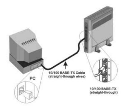
You can connect the Router directly to a 10/100BASE-TX Ethernet adapter card (NIC) installed on a PC using the Ethernet cable provided as shown in this diagram.
