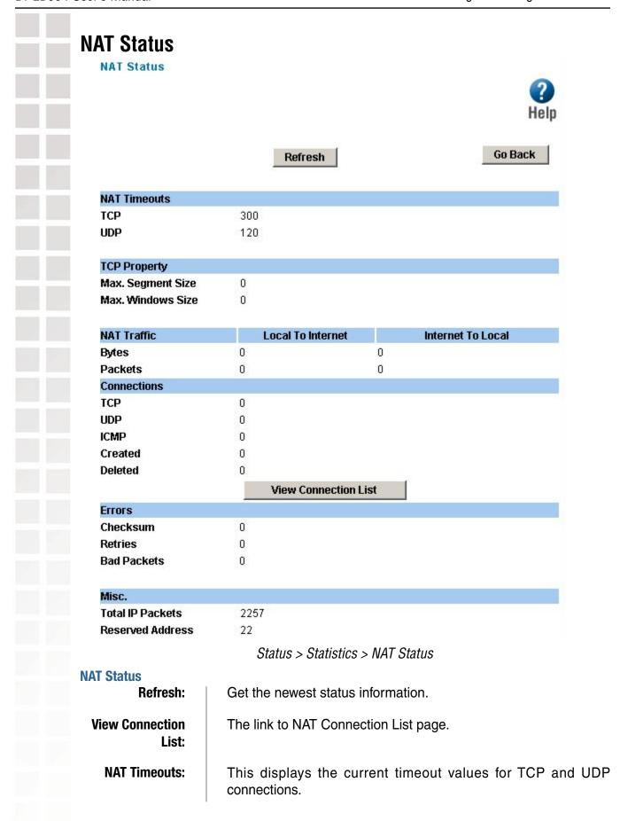
**TCP Property:** This displays the MSS (Maximum Segment Size) and Maximum
