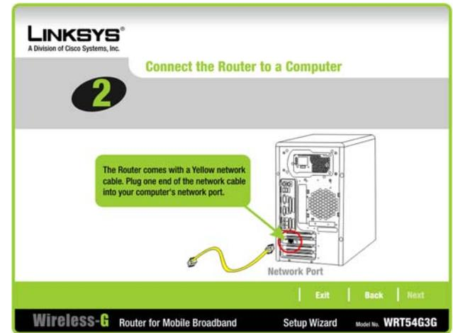
Figure 5-4: Connect the Router to a Computer Screen
