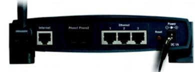
**Figure 4-4: Connect the Power**
