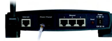
**Figure 4-2: Connect a Telephone**
