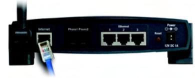
**Figure 4-3: Connect the Modem**
