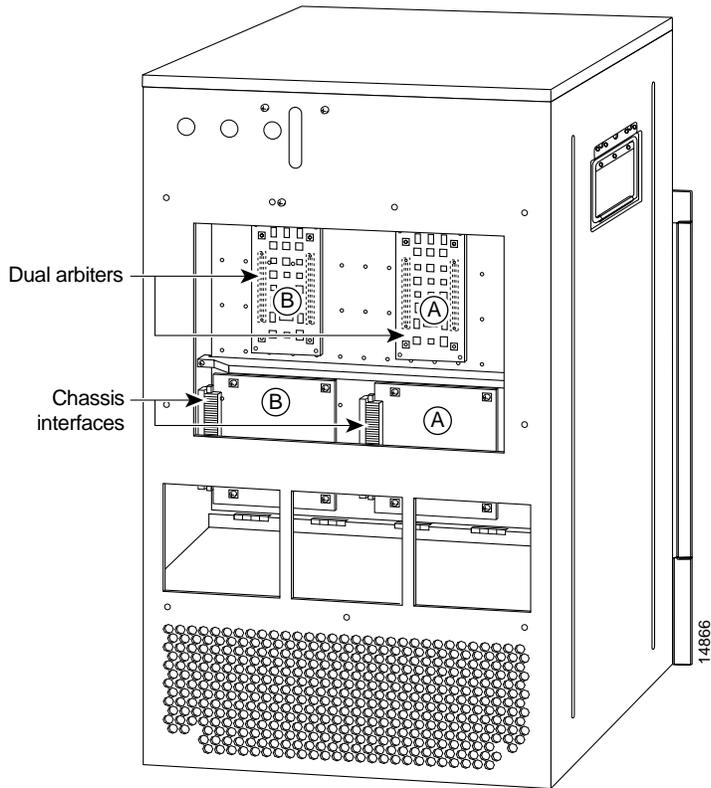
**Note** When you view the rear of the card cage, the dual arbiter and chassis interface on the right side are used with router A, and the dual arbiter and chassis interface on the left side are used with router B.
