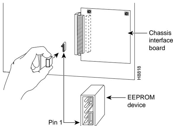
**Figure 13** Location of the EEPROM Devices on the Rear of the Card Cage (Cisco 7576)
