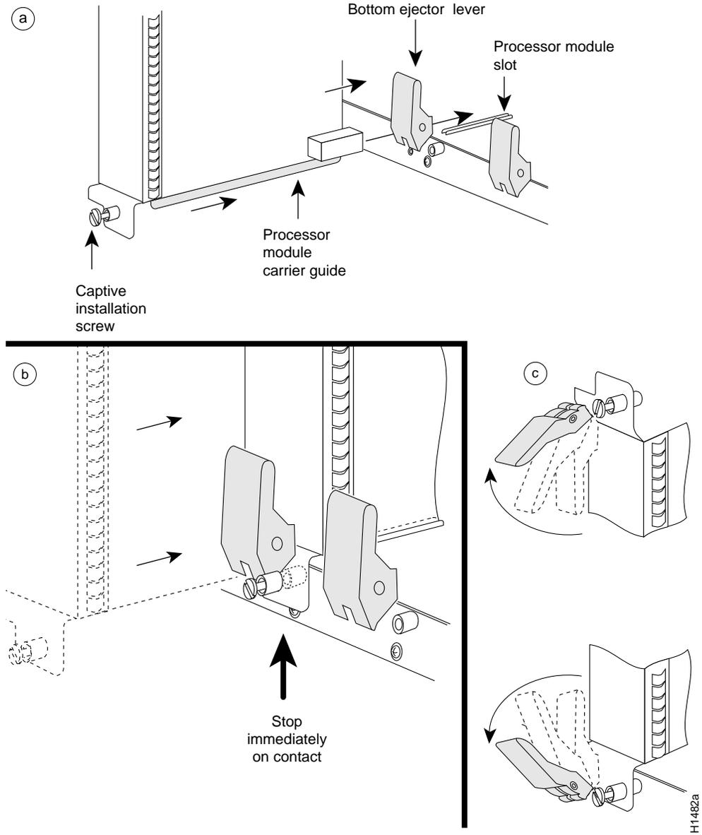
Figure 6 Board Rack with Processor Modules
