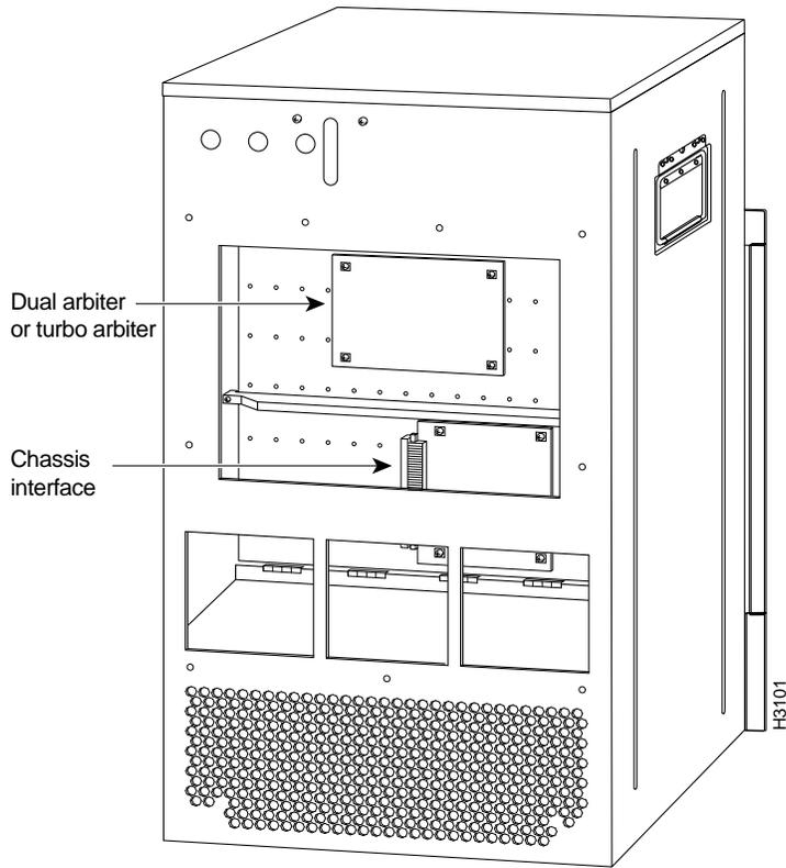
Figure 4 shows the location of the Cisco 7576 dual arbiters and chassis interfaces on the rear of the backplane.
