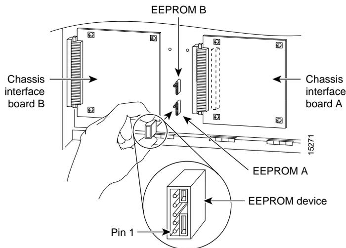
**Note** The Cisco 7576 features two routers on one backplane. These are designated router A and router B. The backplane of the Cisco 7576 includes two dual arbiters, two chassis interfaces, and two EEPROM devices. Figure 13 shows the specific location and designation of each EEPROM device.
