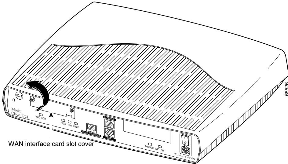
**Step 3** Hold the WIC by the edges on either side of the card front panel, and line up the card edges with the guides inside the card slot, as shown in Figure 4.
