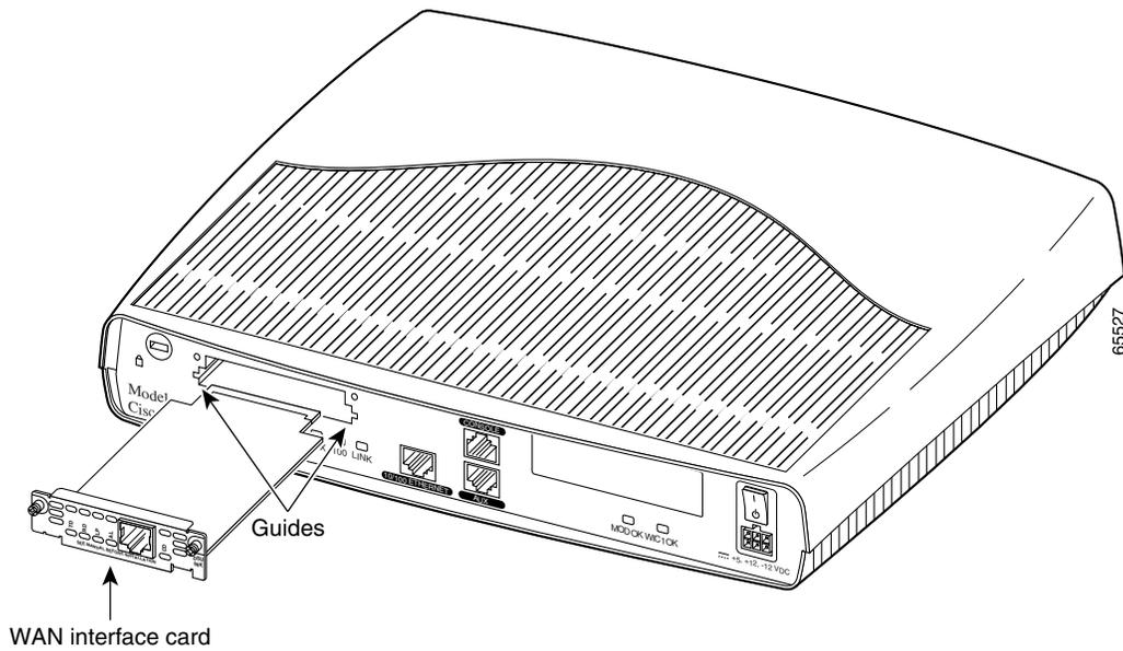
**Step 4** Insert the card in the slot. Gently push it into the router until the front panel of the card is flush with the back panel of the router.
