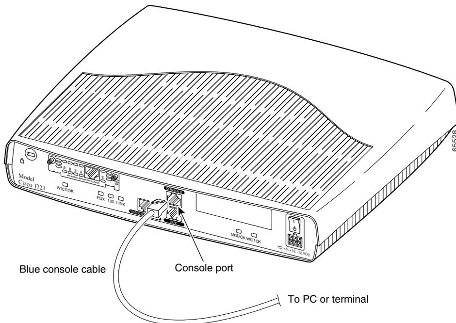
**Step 2** Connect the DB-9 end of the console cable to the console port (also called the *serial port*) on your PC. If this adapter does not fit your PC console port, you must provide an adapter that fits.
