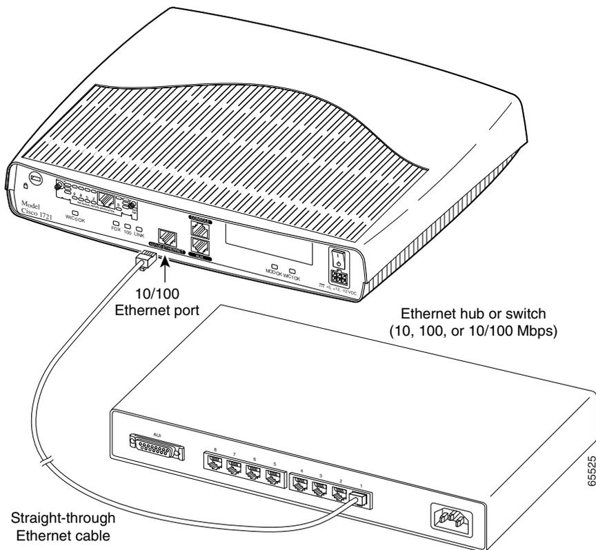
**Step 2** Connect the other end of the cable to a port on the hub or switch.
