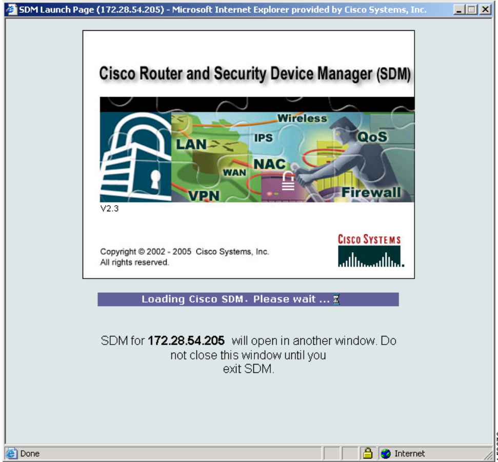
Figure 7 Cisco Router and Security Device Manager (SDM) Launch Screen
