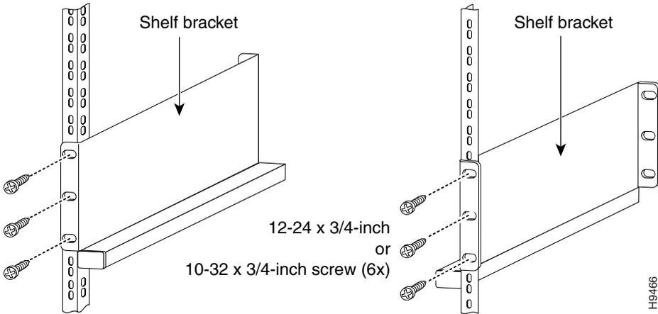
**Figure 3-2** *Attaching the Crossbar Bracket to the Shelf Brackets*
