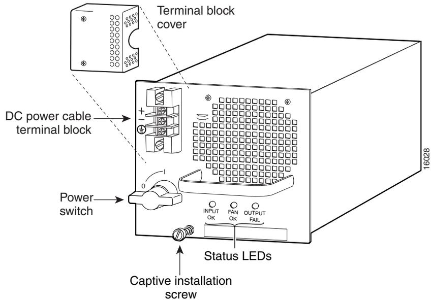
**Step 4** Disconnect the DC-input wires from the terminal block (see [Figure 5-4](#)) in the following order:
