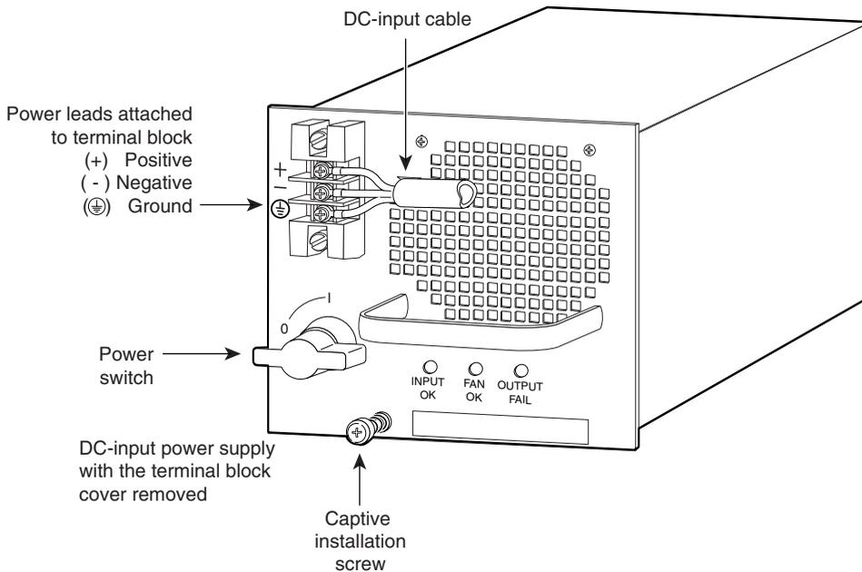
**Step 9** After ensuring that all wire connections are secure, reinstall the terminal block cover.
