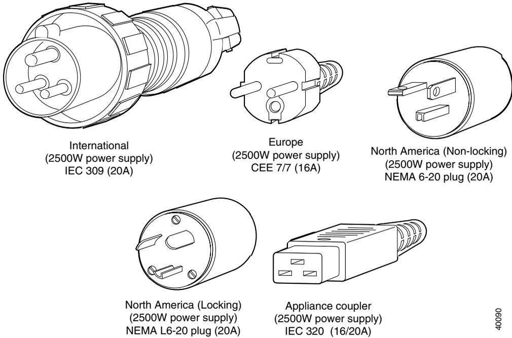
**Figure 2-2 AC Power Cord Connectors for the 4000W Power Supply**
