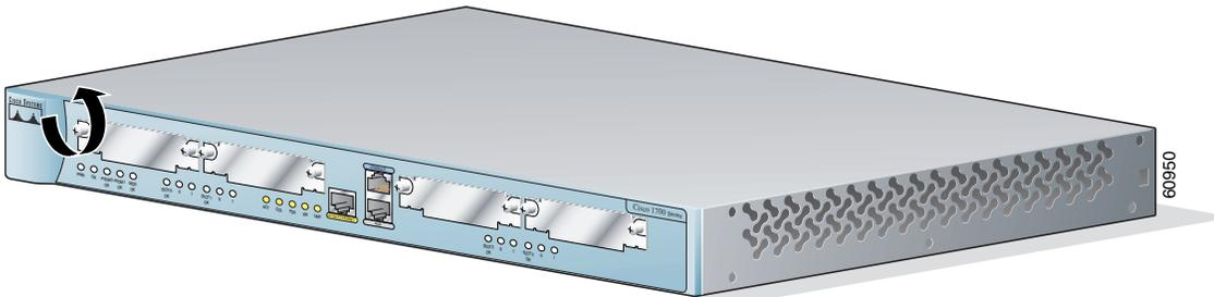
You should be able to loosen the screws using your fingers; however, if the screws are very tight, you may need to use a Phillips screwdriver.
