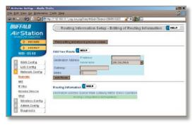
To configure a route manually, enter its *destination address* and *gateway*. Enter a maximum number of hops allowable in *Metric* and click *Add*.
