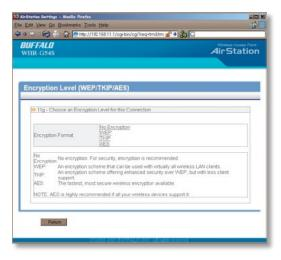
This page is available from *Home* by selecting *Wireless Encryption*. Here, you can manually select the type of wireless encryption you'd like to use. Your AirStation supports three different encryption schemes; choose the best one that all your clients support.
