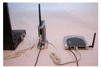
\* Note: Each AirStation may be part of 6 different bridges. Remember that each layer of bridges takes about half your total network speed, so avoid configuring daisy-chains more than 4 bridges long. A star-pattern is always better, with a central router serving multiple bridges.
