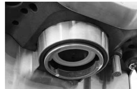
7. Re-insert the dispersion plate, then the shower screen, then the screw. With your fingers, turn the screw clockwise for 2-3 revolutions then insert the Allen Key to tighten until the screw is flush with the shower screen.
