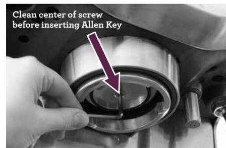
5. Once loosened, carefully remove and retain the screw, stainless steel shower screen and black dispersion plate. Make note of the side of the shower screen and dispersion plate that are facing downwards. This will make re-assembly easier. Wash the shower screen and dispersion plate in warm soapy water, then dry thoroughly.
