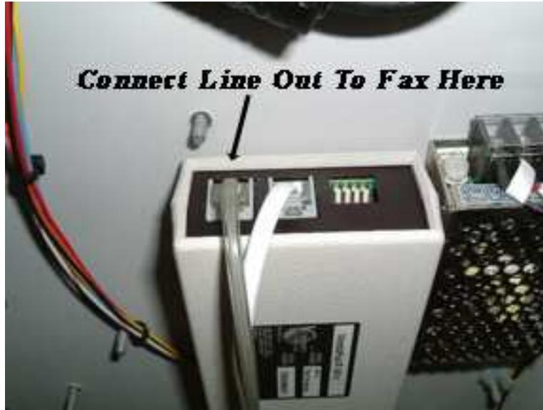
Next, connect the other end of the “To Fax” line to the “Line” jack on your fax device.
