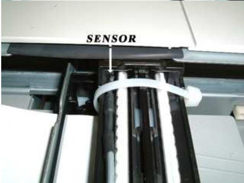
Please note the sensor is held in place with a small ty wrap provided for you in the kit. The ty wrap must be installed in such a way that it does not drag or rub anywhere.
