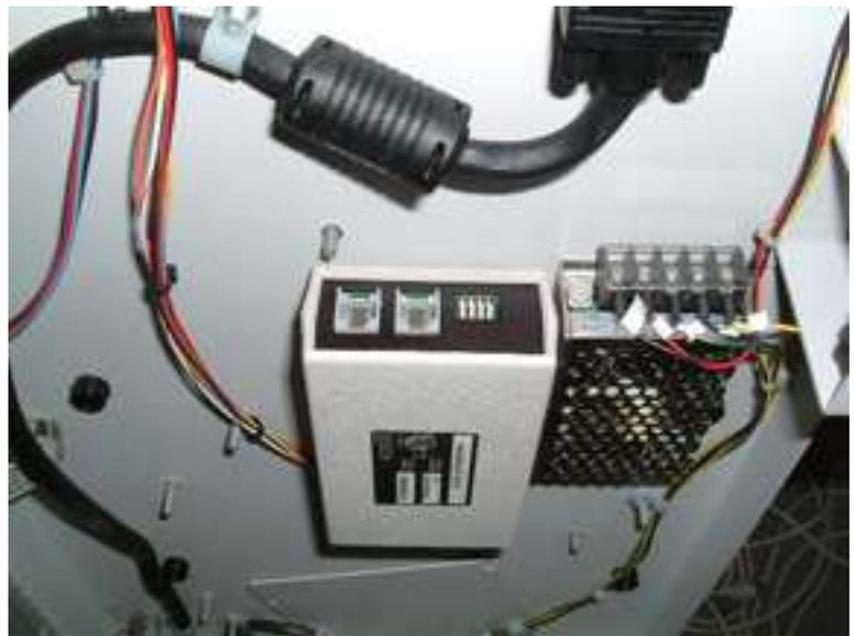
Please note the connections for the Telco Line In and To Fax are pointing up in the enclosure. There is a diagnostic LED next to the switch array that must easily be seen for diagnostics. This also makes the switches easy to get to for programming.
