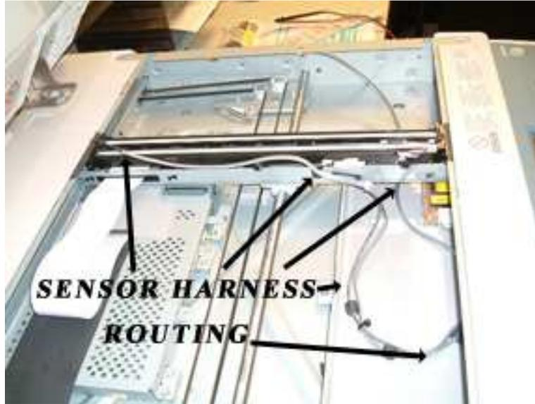
Please note there is plenty of slack in the cable to allow for smooth operation of the scanner light bar. Also note the sensor harness runs UNDER the light bar to exit the copier. Here is a photo of the harness routing on a Samsung C8380ND
