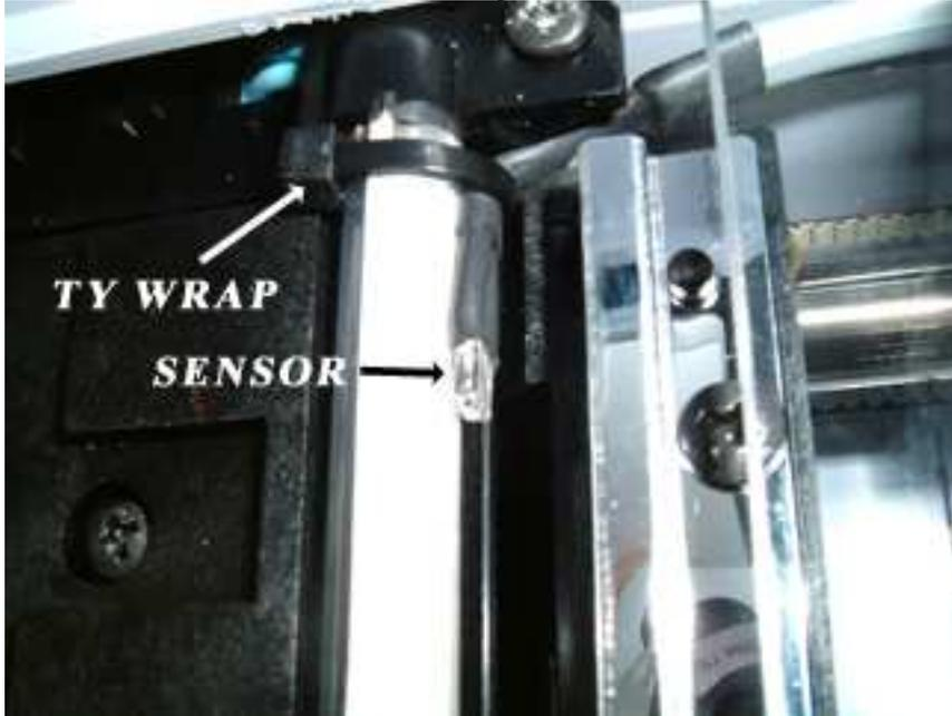
Use caution when installing the sensor so that it does not interfere with the normal operation of the copier
