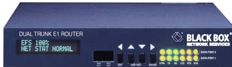
Figure 1-1 Dual Trunk E1 Router
