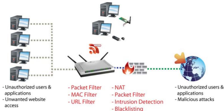
1. **Firewall:** Prevents access from outside your network. The router provides three levels of security support:
