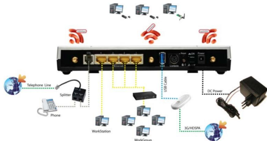
Once you've checked all the connections and you've switched on the Router the product will carry on immediately a diagnosis (about 10 seconds). Finished this, the Led **PWR** will be fixed green and **LAN** and **Wireless** will blink green; DSL will blink during synchronization, and will be fixed when ADSL line is synchronized with WebShare Router. If Led DSL blink continuously, please contact Your ISP in order to check ADSL line state.
