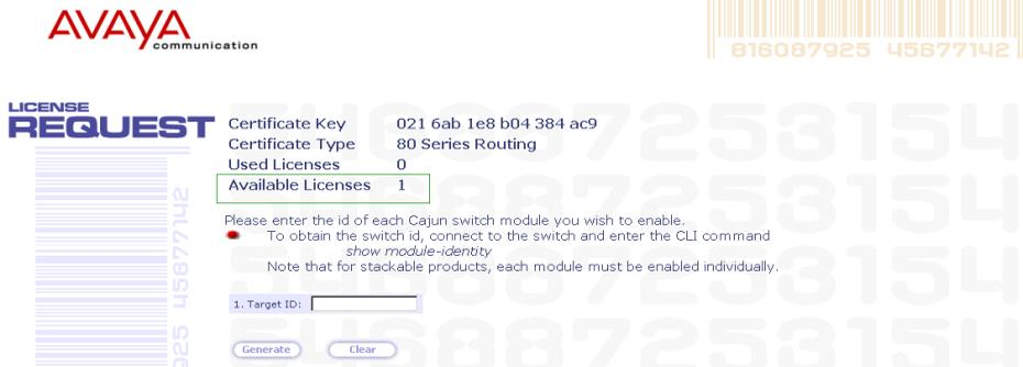
7 Enter serial number of the switch(es) or module. To identify serial numbers use the CLI command:show module-identity.
