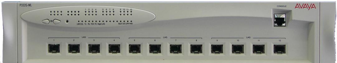
Figure 6.2 P332G-ML LEDs
