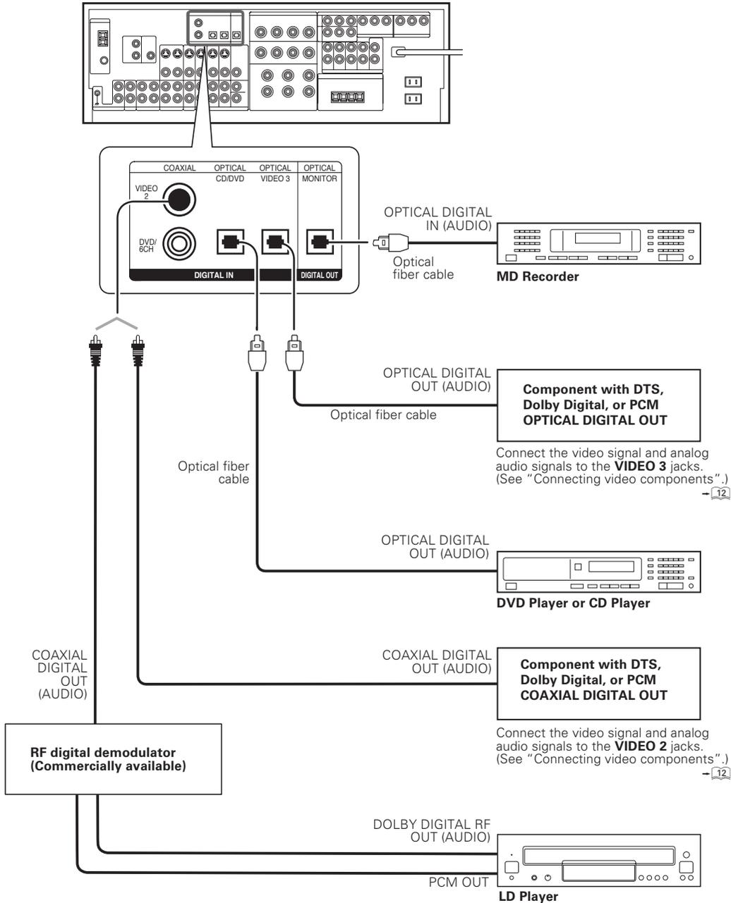
To connect an LD player with a DIGITAL RF OUT, connect the LD player to a RF digital demodulator (commercially available). Next, connect the DIGITAL OUT jacks of the demodulator to the DIGITAL IN jacks of the receiver. Connect the video signal and analog audio signals to the VIDEO 2 or VIDEO 3 jacks. (See "Connecting video components".)
