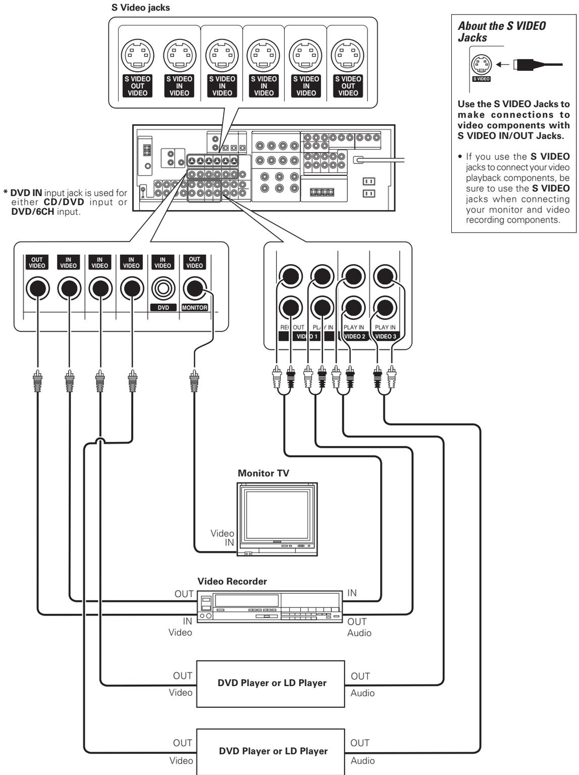
A video component with digital audio outputs should be connected to the VIDEO 2 or VIDEO 3 jacks.
