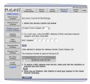
To delete a MAC address, select the corresponding checkbox and click the **Del** button. The maximum number of entries allowed in the table is 32.
