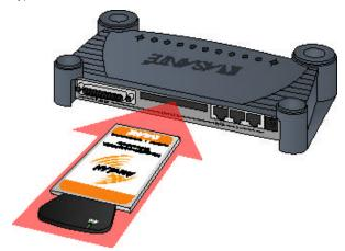
**Note**: The card must be installed before powering up your computer or router.
