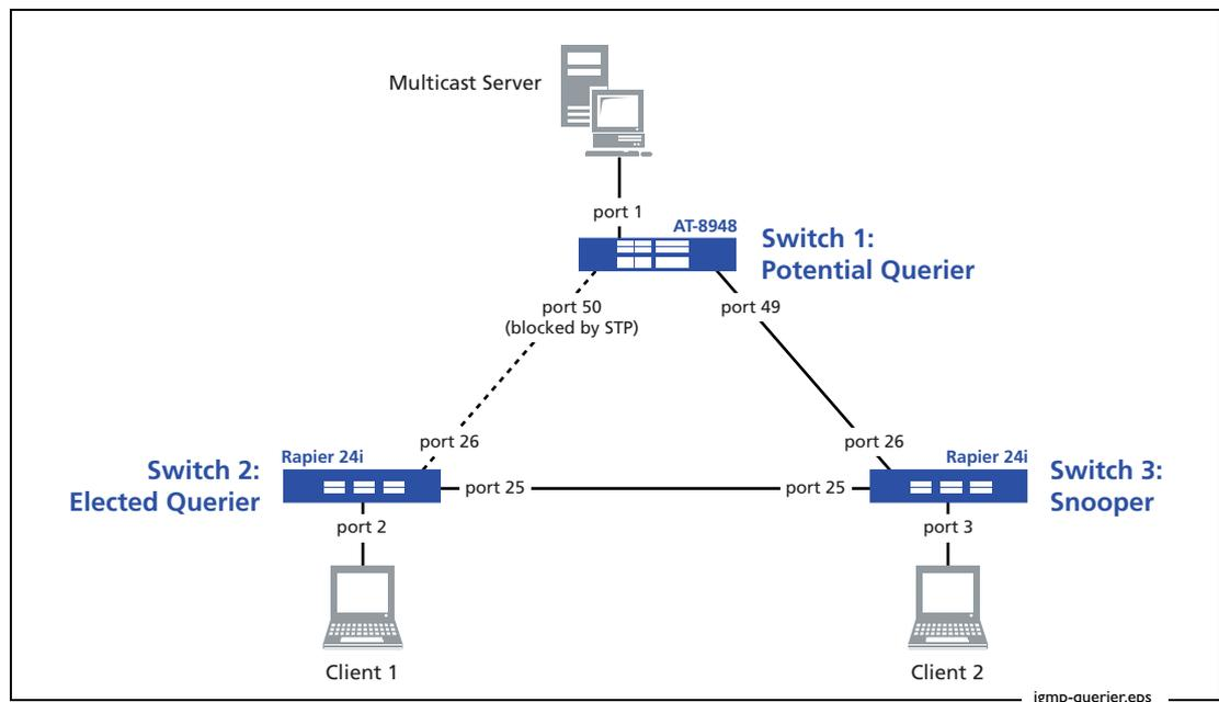
Both switch 1 and switch 2 are configured with IGMP, making both of them potential Queriers. Switch 3, by default configuration, is an IGMP Snooper.
