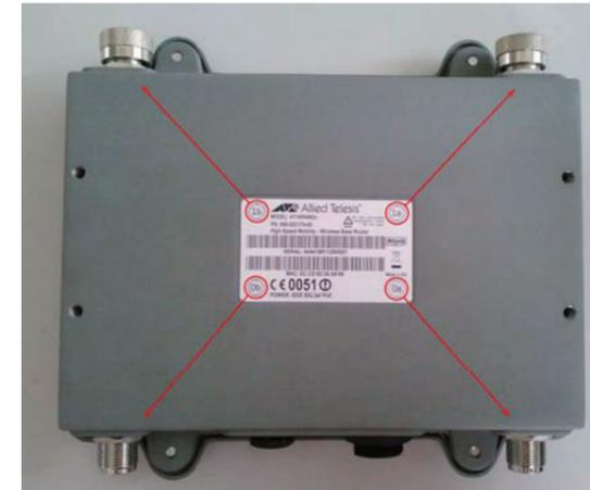
Figure 1: AT-WR4662n antenna connectors
