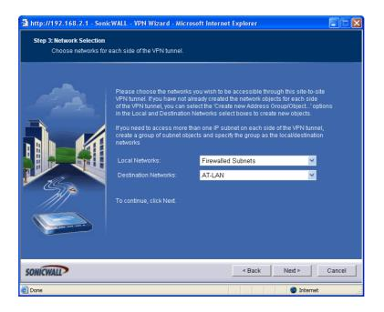
For the local (SonicWALL) end, select Firewalled Subnets. For the destination (Allied Telesis) end, select the address object that you created in "Define the LAN subnet of the peer" on page 20.
