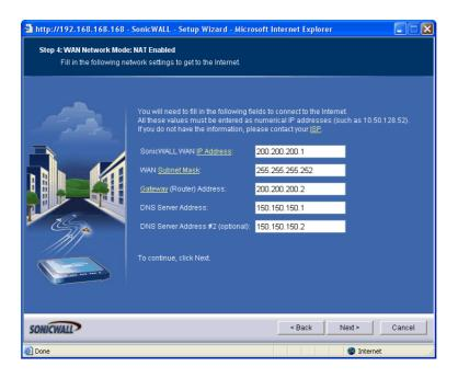
Enter the WAN interface's IP address and mask. For Gateway, enter the ISP's address (see "The network" on page 3). For DNS Server Address, enter the address of the DNS server that your router will access.
