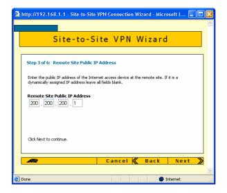
Enter the public IP address of the other end of the tunnel. In this example, this is 200.200.200.1, which is the IP address of the SonicWALL WAN interface.
