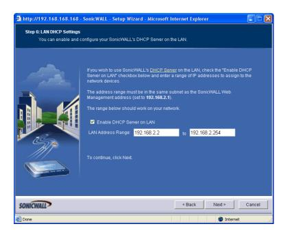
In this step, you can set up the DHCP server on this router to service the office LAN you intend to connect to. Check that the wizard has chosen an appropriate range of addresses.
