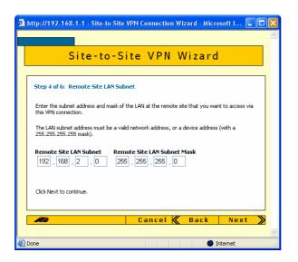
Enter the SonicWALL router's LAN subnet address and mask. In this example, this is 192.168.2.0 and a mask of 255.255.255.0.
