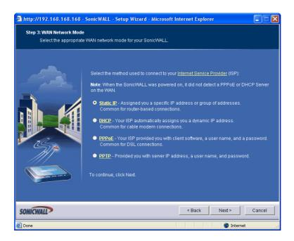
In this example, the SonicWALL router has a permanent fixed IP address, so select the Static IP option.
