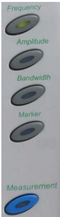
**Frequency:** Use this key for accessing the frequency menus. The frequency menus allow you to set the center, start, and stop frequencies, frequency span, frequency step size, and frequency offset. The default parameter is the center frequency.
