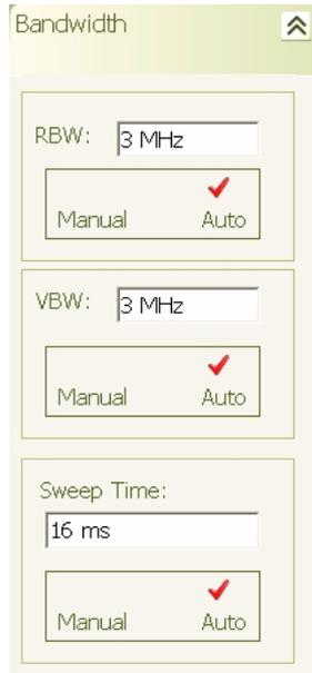
The screenshot shows the 'Bandwidth' menu with three sections. Each section has a text input field and a radio button selection. The 'RBW' section has '3 MHz' in the field and 'Auto' selected. The 'VBW' section has '3 MHz' in the field and 'Auto' selected. The 'Sweep Time' section has '16 ms' in the field and 'Auto' selected.
