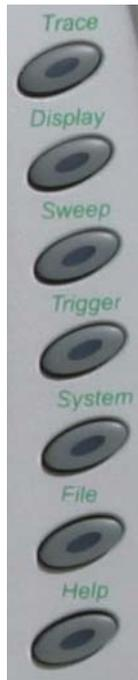
**Trace:** Use this key for accessing the trace menus. The trace menus are used to set the active trace, select the trace state, set the number of averages for the trace display, and to select the detector type. The default parameter is the active trace selection.
