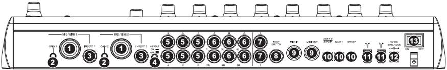
1. **MIC / LINE INPUTS** – These two inputs can accept microphones (using an XLR cable) or an instrument or line-level device (using a 1/4" cable) such as a guitar, bass, sampler, or other audio device. These are balanced, low-impedance inputs. For best results when connecting balanced, line-level gear, use a TRS (tip-ring-sleeve) cable to connect to the 1/4" inputs.
