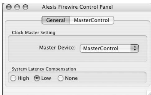
**1. Master Device:** Ensure that your MasterControl is an option in this drop-down box. If the MasterControl is not shown, then your computer does not “see” it. Check the mixer’s connection to your computer.
