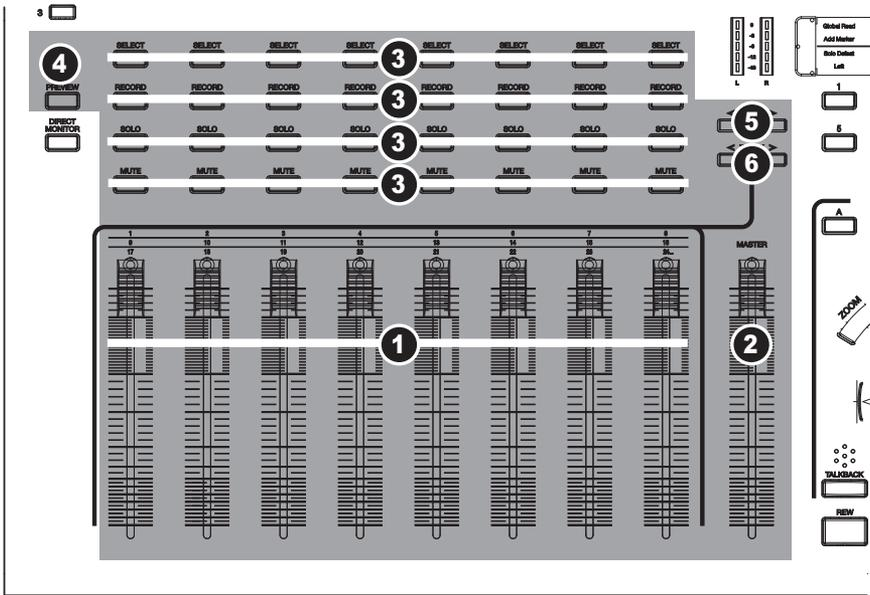
1. **CHANNEL FADER** – Use this 100mm, touch-sensitive fader to adjust the volume levels of each channel. The exact level will be shown in the DISPLAY.
