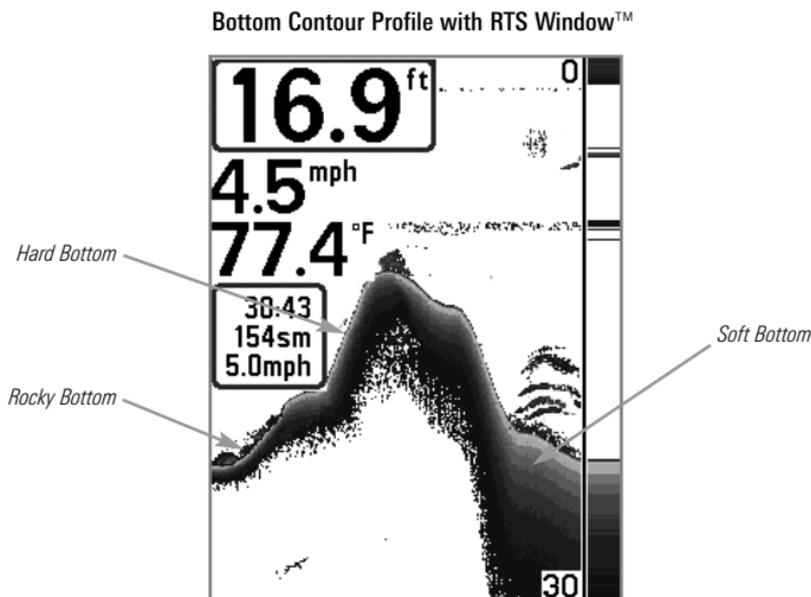
The sonar returns from the bottom, structure, and fish can be represented as **Inverse**, **Structure ID®**, **WhiteLine™**, or **Black** (Bottom Black). See *Sonar X-Press™ Menu: Bottom View* to set the bottom view.
