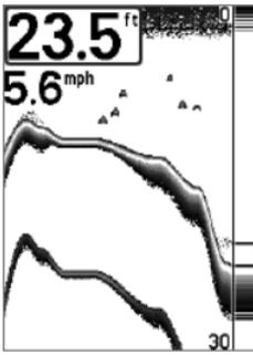
**Inverse** is a method where weak returns are shown with dark pixels and strong returns with lighter pixels. This has the benefit of ensuring that weak signals will be clearly visible on the display.
