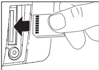
Inserting an MMC/SD
