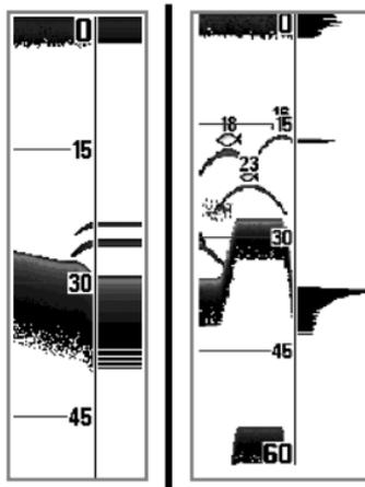
The **Wide RTS Window™** indicates the sonar intensity through the use of a bar graph. The length of the plotted return indicates whether the return is weak or strong. The depth of the sonar return is indicated by the vertical placement of the return on the display depth scale. The Wide RTS Window™ does not use grayscale.
