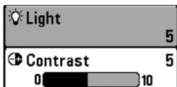
**Adjust the Backlight or the Display Contrast:** Press the POWER/LIGHT key to access the Light and Contrast submenu. Use the 4-WAY Cursor Control key to select Light or Contrast, and then use the LEFT or RIGHT Cursor key to change the settings. Press EXIT to exit the Light and Contrast submenu.
