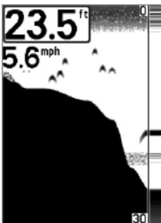
**Black (Bottom Black)** displays all pixels below the bottom contour as black, regardless of signal strength. This has the benefit of providing a high contrast between the bottom and other sonar returns on the display.
