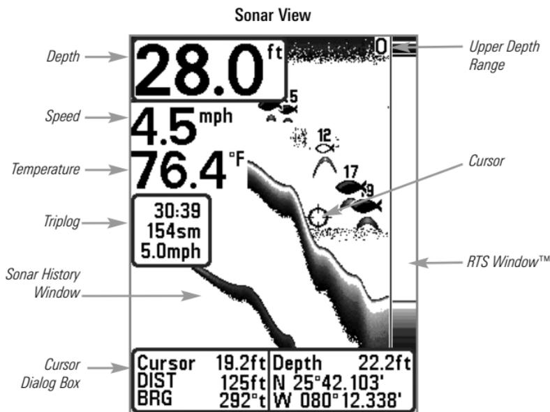
**NOTE:** If the Depth number is flashing, it means that the unit is having trouble locating the bottom. This usually happens if the water is too deep, the transducer is out of the water, the boat is moving too fast, or for any other reason that the unit can't accurately receive continuous data.
