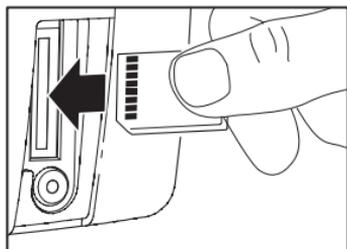
Inserting an MMC/SD
