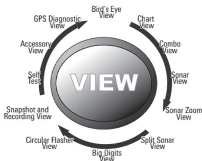
The sonar and navigation information from your Fishfinder are displayed on the screen in a variety of easy-to-read views. There are many views available on your Fishfinder. When you press the VIEW key, the display cycles through the available views on your screen. When you press the EXIT key, the display cycles through the available views in reverse order.
