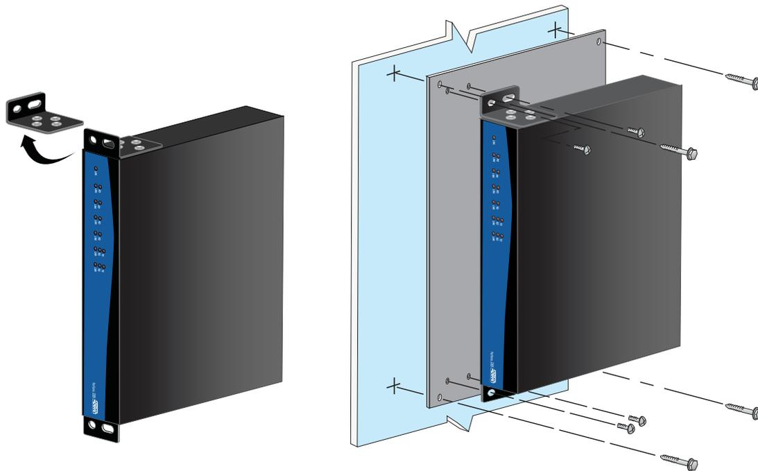
Figure 30. Repositioning the Mounting Bracket for Wall Mounting the NetVanta 3205/3305
