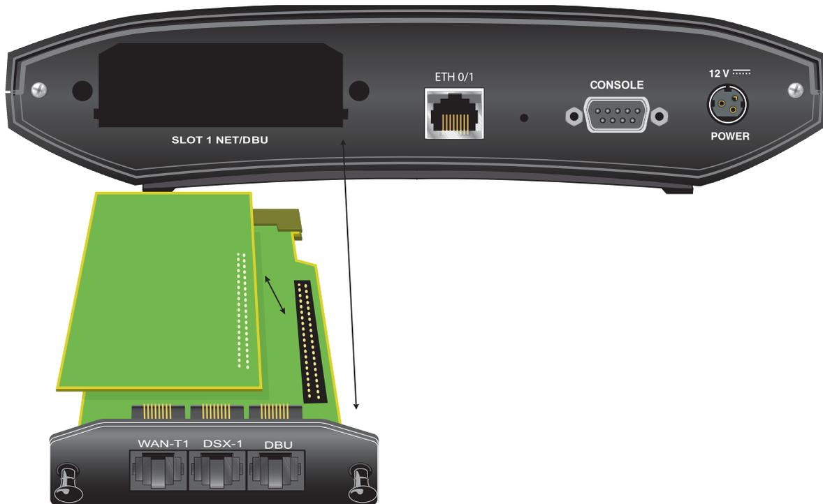
Figure 37. NIM and DIM Installation
