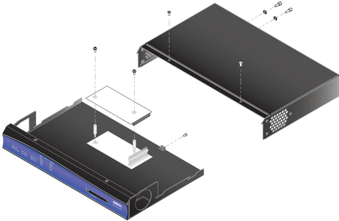
**Figure 43. NetVanta Octal PoE Upgrade Installation**
