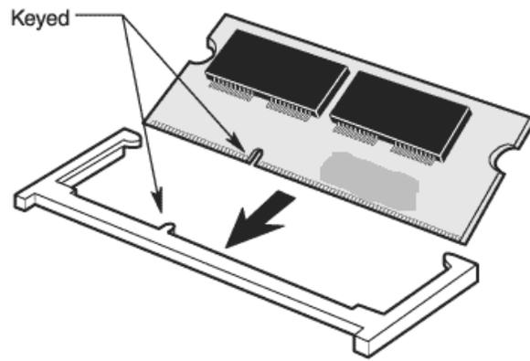
**Figure 39. SODIMM Installation – Keyed Slots**
