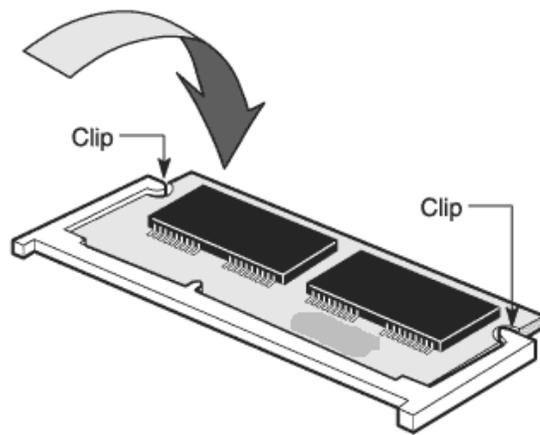
**Figure 41. SODIMM Installation – Rotating the Module Downward**
