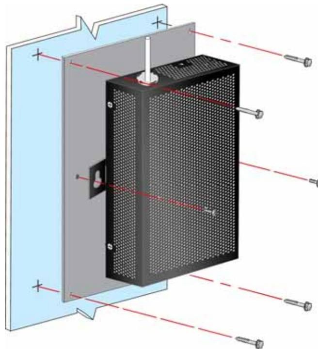
**Figure 33. Wall Mounting the NetVanta PoE Power Supply**
