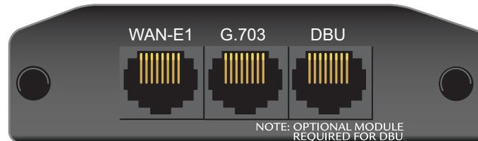
**Figure 22. NetVanta E1/FE1 + G.703 NIM**
