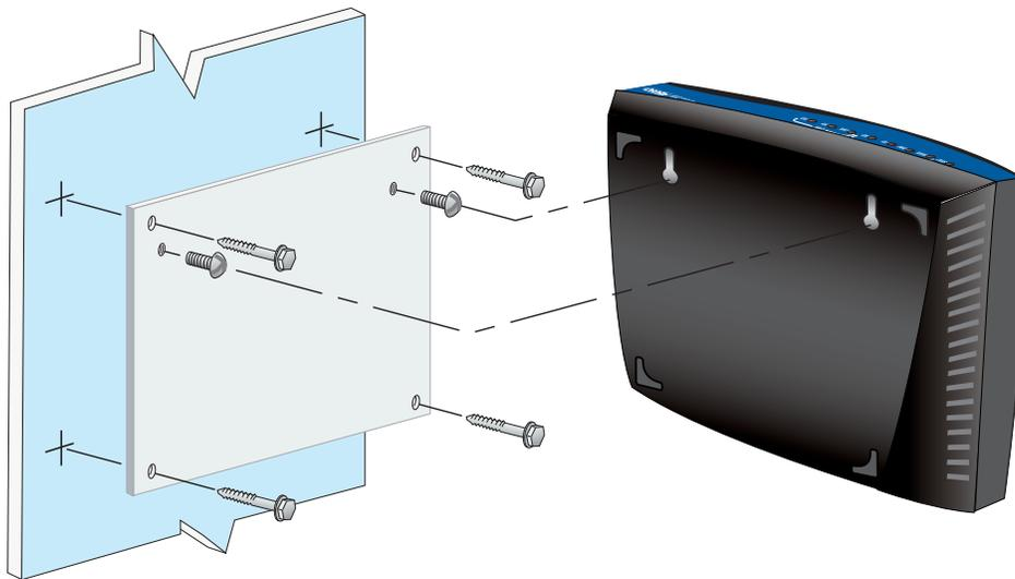
Figure 29. Wall Mounting the NetVanta 3200
