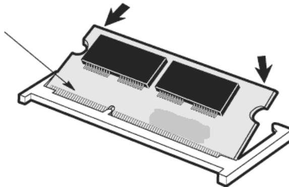
**Figure 40. SODIMM Installation – Applying Pressure**
