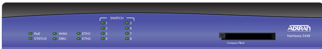
**Figure 10. NetVanta 3448 Front Panel Layout**
