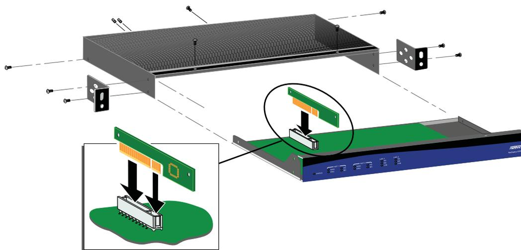
**Figure 38. NetVanta VPN Accelerator Card Installation**
