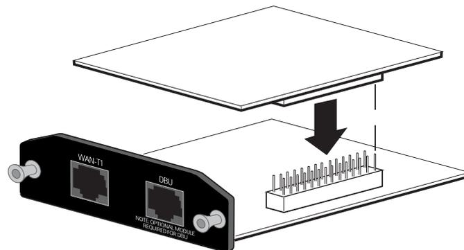
Figure 36. Installing DIMs
