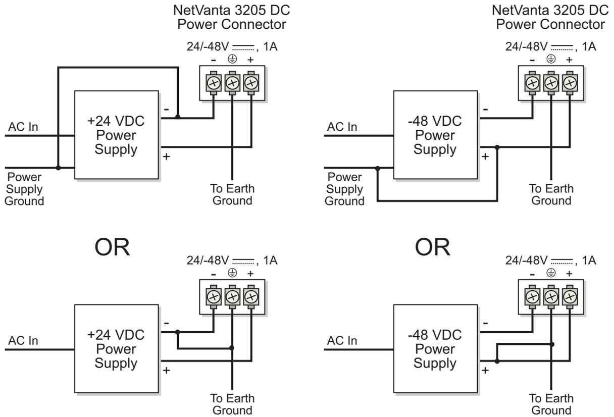
**Figure 35. NetVanta 3205 DC Power Connection**
