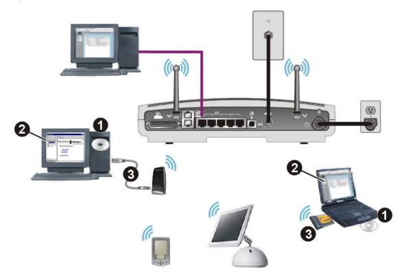
To set up the SBG1000, on a computer wired to the SBG1000 over Ethernet or USB, perform the procedures in "Setting Up the Wireless LAN". Do not attempt to configure the SBG1000 over a wireless connection.
