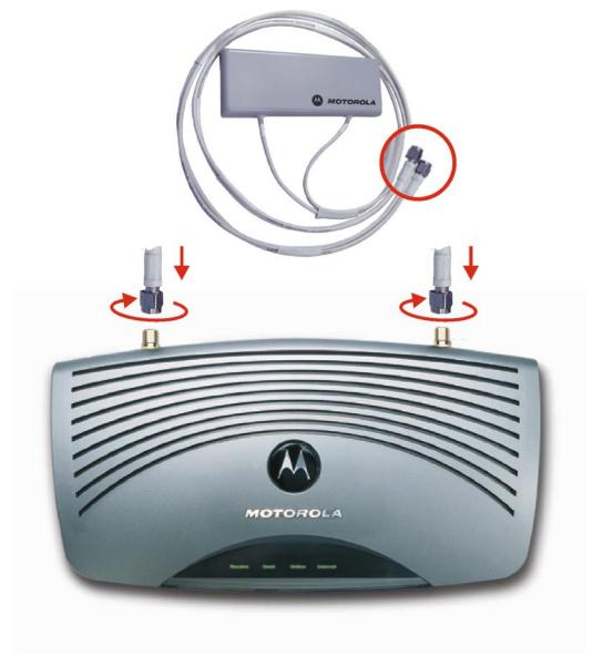
Position or mount the External Diversity Antenna in a suitable location away from the computer and monitor. Follow the instructions provided with the External Diversity Antenna. Do not twist the antenna cables.
