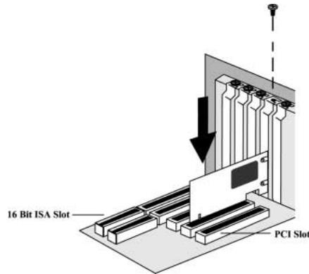
2. Carefully insert and secure the modem into an open PCI slot and close the computer.
