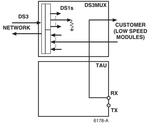
**Figure 575-3b. Drop: None/Insert: Customer**
