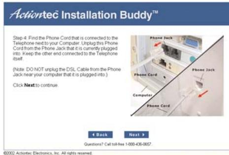
☞ **Note:** Do not remove the DSL Cable from the phone jack near the computer.
