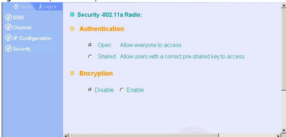
*Authentication Type* – Use “Open System” to allow open access to all wireless clients without performing authentication, or “Shared Key” to perform authentication based on a shared key that has been distributed to all stations. (Default: Open System)
