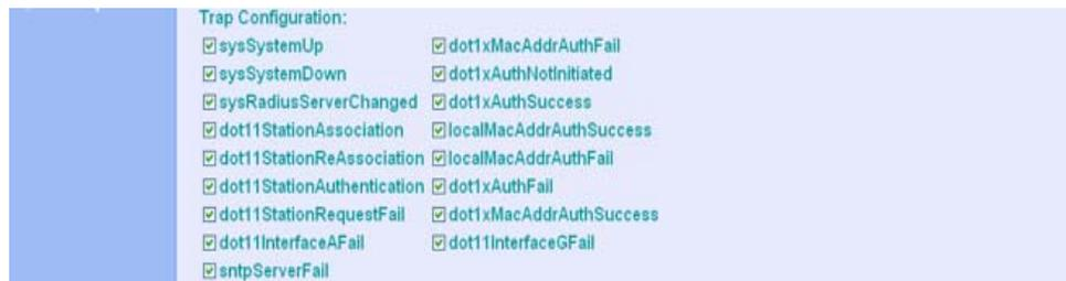
*Trap Configuration* – Allows selection of specific SNMP notifications to send. The following items are available:
