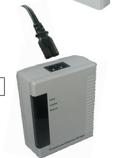
Plug the other end of this cable into an electrical socket.
