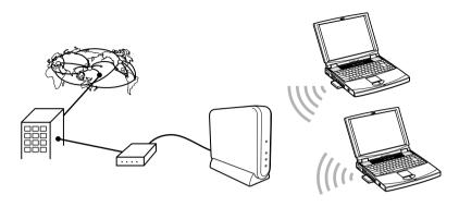
1 Connect the DSL modem and the Access Point with an Ethernet cable.
