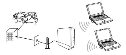
1 Connect the ISDN router and the Access Point with an Ethernet cable.
