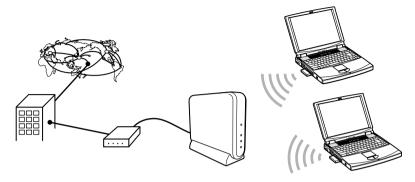
**1** Connect the cable modem and the Access Point with an Ethernet cable.
