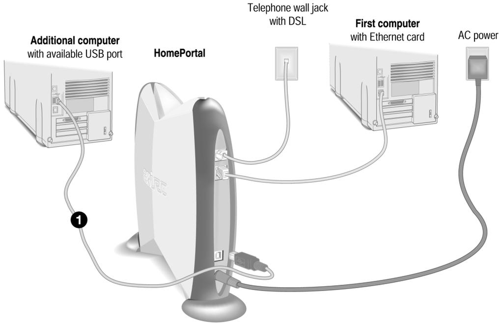
**Note:** In a HomePortal network, only one Windows 98, 98 SE, Windows ME, Windows 2000, or Windows XP computer can be directly connected to the HomePortal residential gateway using the USB connection. Additional computers may be added to the network using connection options such as Ethernet. HomePortal USB connectivity is not available for Macintosh, Windows 95, Windows 95 OSR2, or Windows NT.
