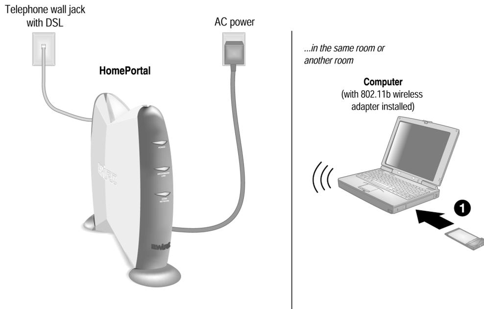
**Note:** If you use a 2Wire wireless adapter (PC card or USB adapter) for wireless networking, the HomePortal Setup Wizard software automatically configures it to communicate with the HomePortal during setup, but you will need to install the driver. See Appendix A for detailed installation instructions.
