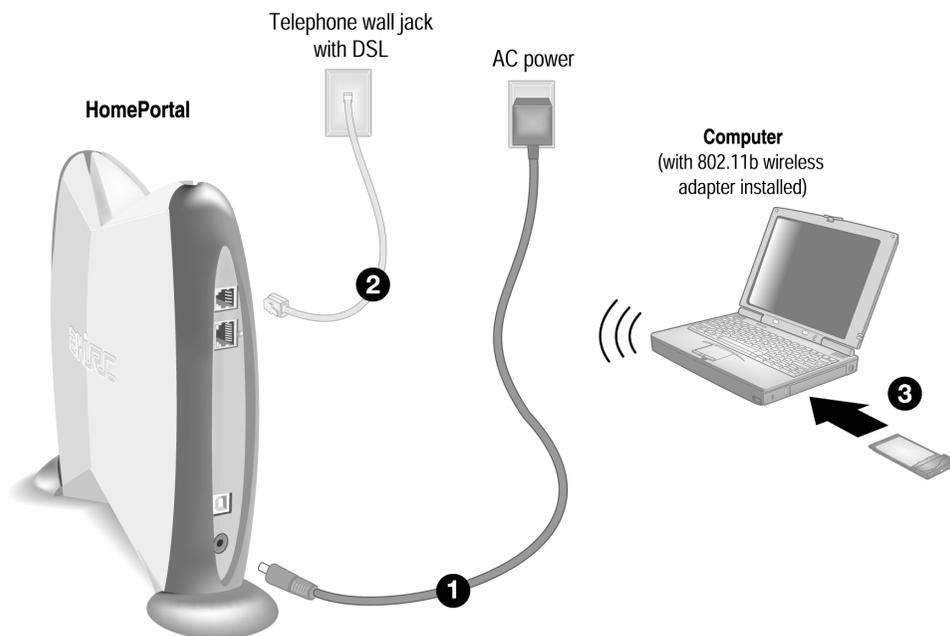
1. Connect the provided AC power adapter from the HomePortal’s **POWER** port to an electrical outlet. The green **POWER** light on the front of the HomePortal should come on.
