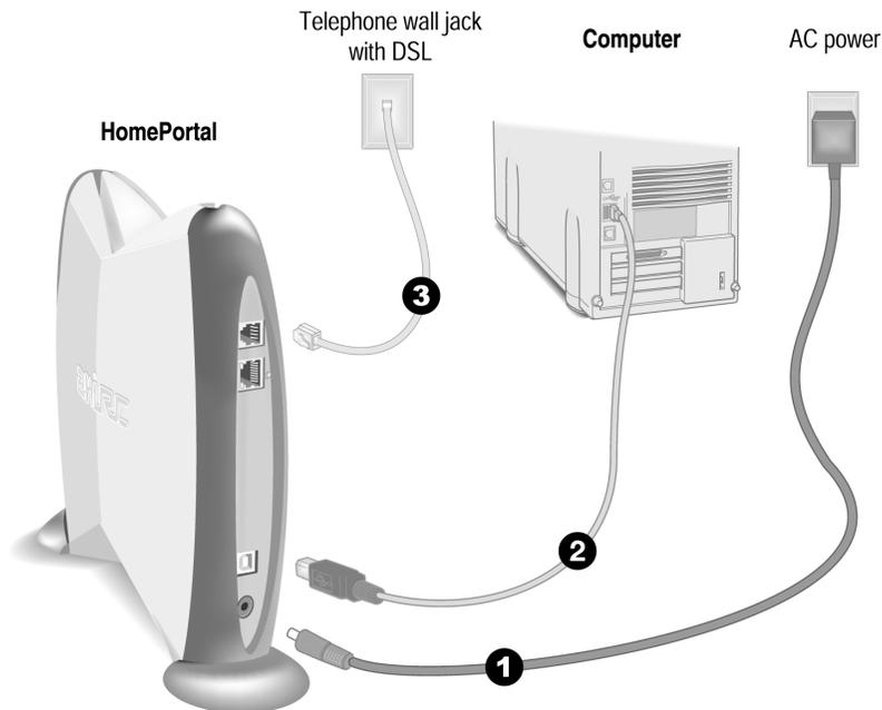
**Note:** In a HomePortal network, only one Windows 98, 98 SE, Windows ME, Windows 2000, or Windows XP computer can be directly connected to the HomePortal residential gateway using the USB connection. Additional computers may be added to the network using connection options such as Ethernet. HomePortal USB connectivity is NOT available for Macintosh, Windows 95, Windows 95 OSR2, or Windows NT.
