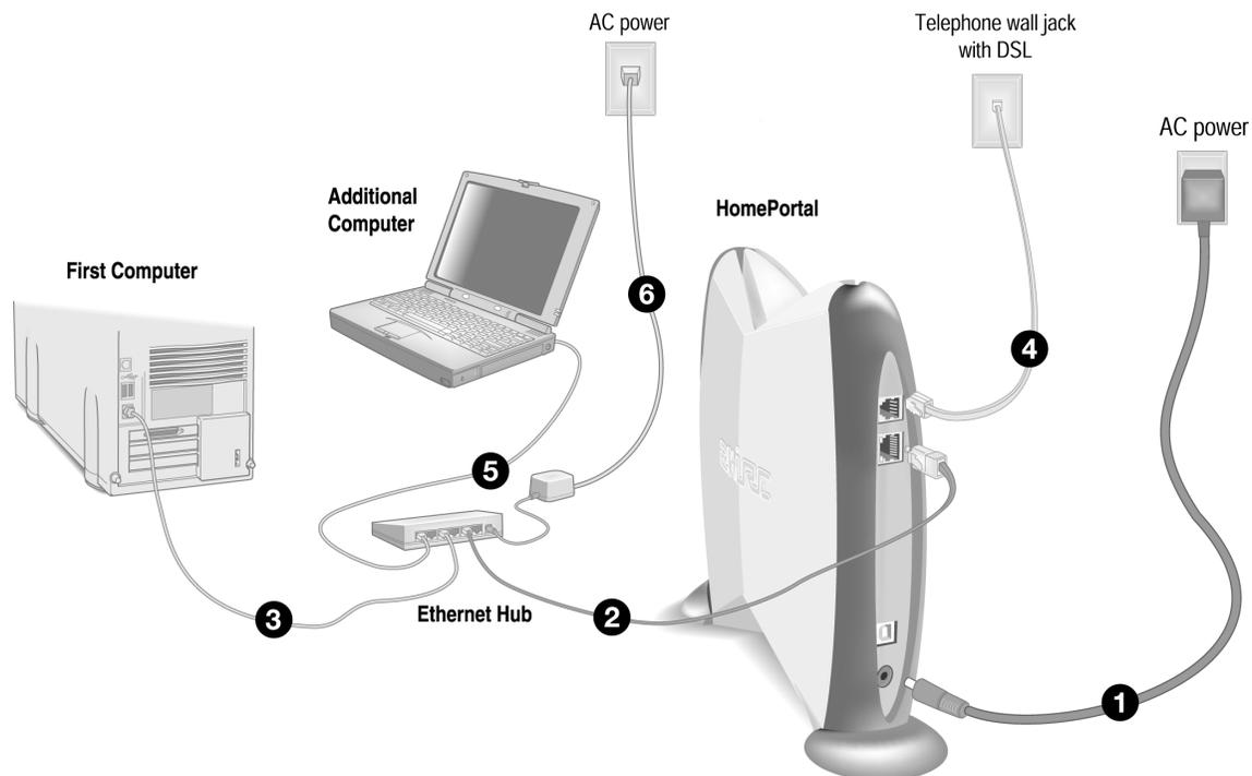
***Note:** The HomePortal has an auto-crossover port. You do not need to use a special crossover cable or make any changes to the configuration of your HomePortal, Ethernet hub, or switch. The HomePortal will establish the type of port needed during setup.*
