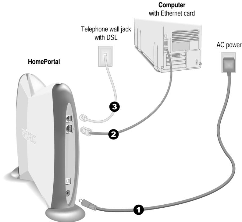
1. Connect the provided AC power adapter from the HomePortal's **POWER** port to an electrical outlet. The green **POWER** light on the front of the HomePortal should come on.
