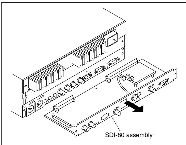
4. Insert the connector (CN601) on the DV-29 board into the connector (CN41) on the SDI-80 assembly.
