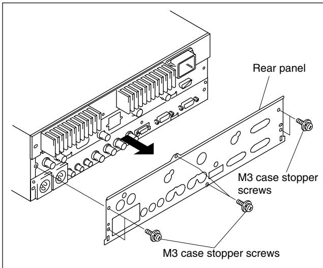
3. Pull out the SDI-80 assembly from the second slot from the bottom of the J-H3 in the direction of the arrow.
