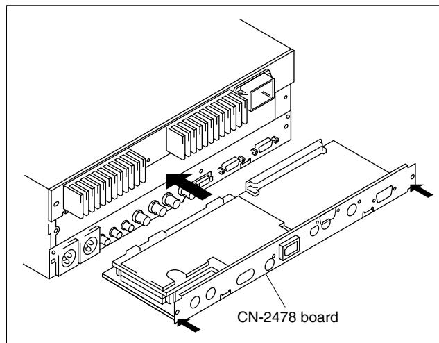
7. Install the supplied rear panel for J-H1 using the six M3 case stopper screws.
