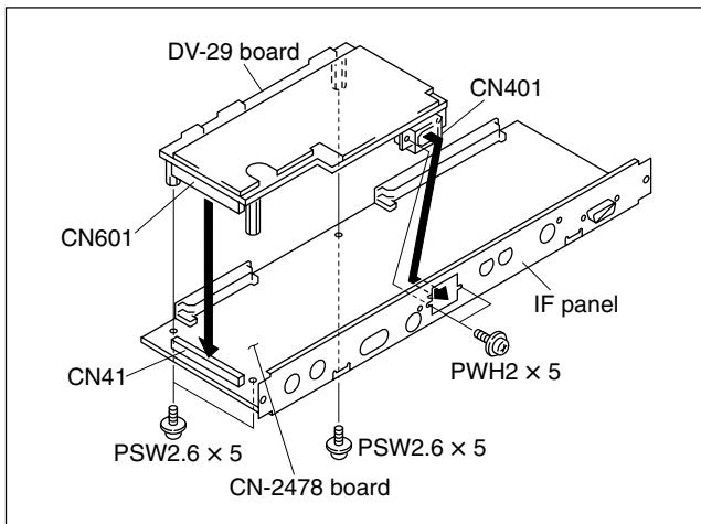
5. Insert the CN-2478 board to the second slot from the bottom of J-H1.
